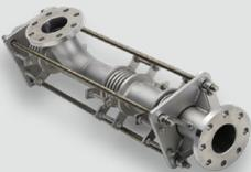
Pressure Balanced Expansion Joints are devices which produce no pressure thrust forces in the piping system on the main anchors. In addition to eliminating the pressure thrust, the expansion joint can accept axial compression, axial extension, lateral and angular movements. The balancing thrust is created by using a balancing bellows.
