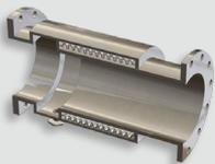
The Externally Pressurized Bellow absorbs a very long stroke that minimizes the number of expansion joints required for a typical installation. Inherent in the design are internal guide rings, a full thickness cover, self-draining convolutions, and an integral liner that is insensitive to the flow direction.
