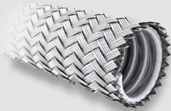
Braid is a sleeve of woven wires that covers the exterior of the corrugated hose. Braid allows the corrugated hose to withstand pressure while providing protection against abrasion and contamination.
