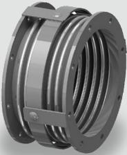
Gimbal Expansion Joints have a single bellow and gimbal hardware designed to resist pressure thrust. The gimbal expansion joint hardware operates like the universal joint on a drive shaft to accommodate angular movements in any plane.
