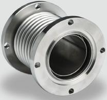
Single Expansion Joints has one bellow. Extension lateral and angular movement can be accommodated. These expansion joints do not restrain the internal pressure thrust. Where small thermal movements are involved and proper anchoring and guiding is feasible, a single expansion joint is the most economical installation.
