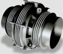
In-Line Pressure Balanced Expansion Joint consists of single or double (universal) bellows to accept the piping induced axial compression, extension and lateral movements. An oversize bellows with approximately two times the area of the flow bellows is used to create an annular pressure chamber that produces a balancing pressure thrust force.
