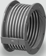
Hinged Expansion Joints have a single bellow with overall length restrained by hinge hardware designed to accommodate pressure thrust.
